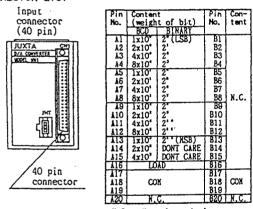
N.C.: Unused terminal LOAD: Load signal
