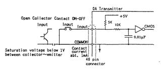
• Resolution Resolution means minimum change of input signal. In case of DA transmitter, minimum resolutions are 1/7999 for BCD input and 1/8191 for BINARY input. In case input range is designated, 1/input span is resolution.
